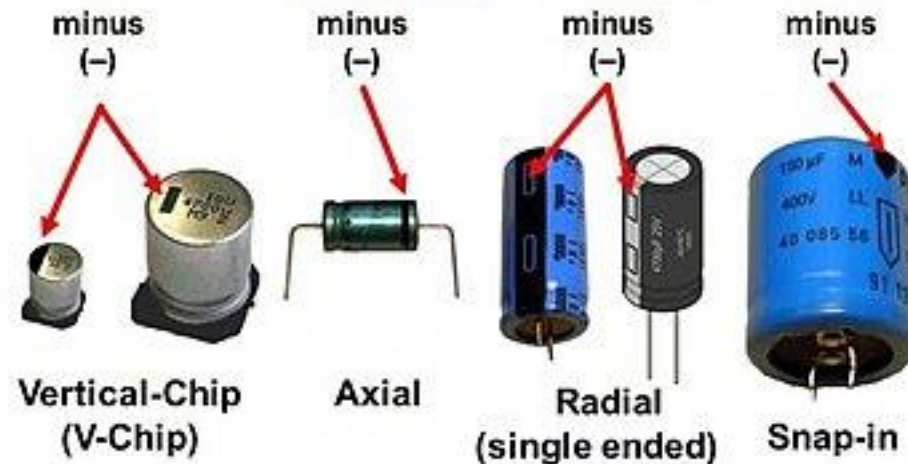
Aluminum electrolytic capacitors with non-solid electrolyte
